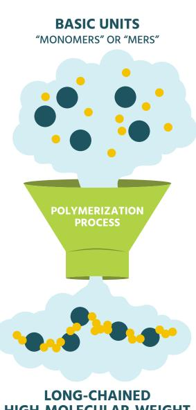
Plastics are made of large numbers of "monomers", which are assembled into long chains called "polymers".
