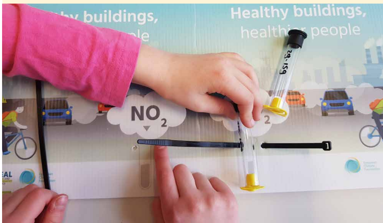
► Citizen science monitoring - children help to set up monitoring tubes for nitrogen dioxide ( \text{NO}_2 ) in the classroom | © HEAL |
