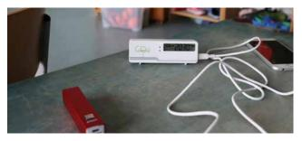
A mini CO<sub>2</sub> monitor was used which contains a traffic light system for classifying the indoor CO<sub>2</sub> concentration.
