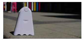
► The low cost air monitor works with a light scattering method to measure fine particulate matter. | © AEEA |
